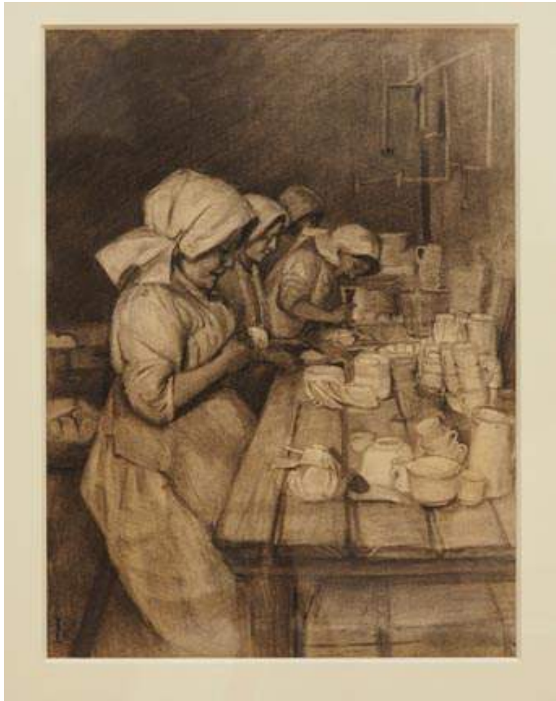
Fig. 7 On a Pot Bank: Scouring and Stamping the Maker's Name on Biscuit China (1907)
